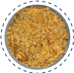
Mycelium promotional items Promising output; friability defects to be neutralized
