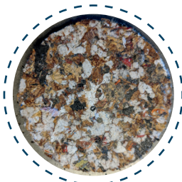
Furniture stuffing (non-woven) Promising, but flammability defect to be neutralized; mechanical tests shall be conducted.
